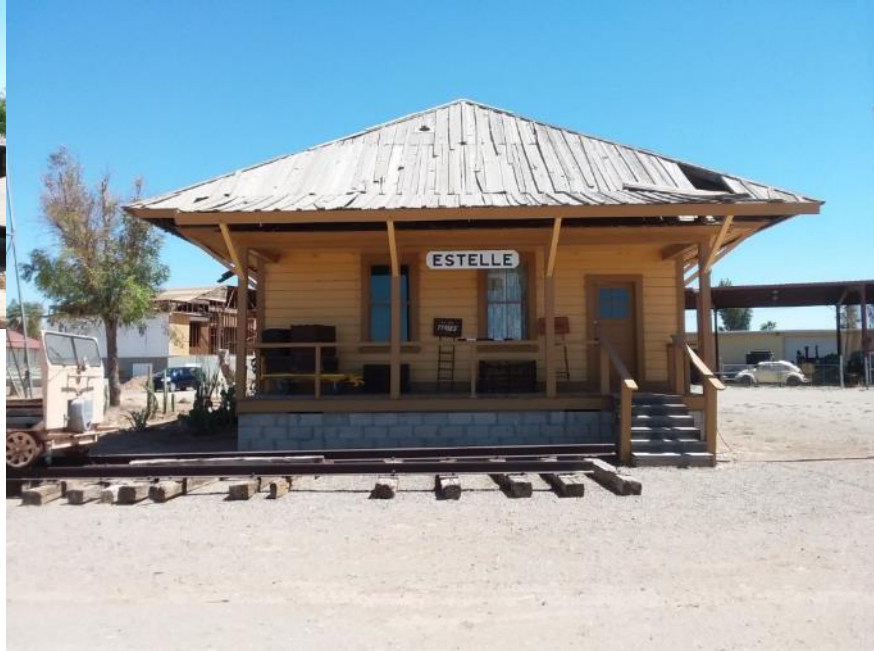
Estelle is about 25 miles north of Imperial but the old depot has been moved to the Pioneers Park Museum. An interesting feature is the double roof. The top roof is a canopy to reduce the effects on the hot sun on the structure.
