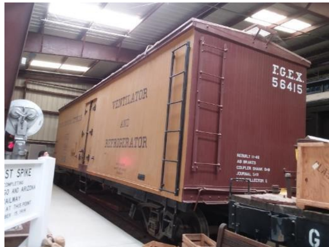
Ice cooled refrigerator cars carried California produce to eastern markets
