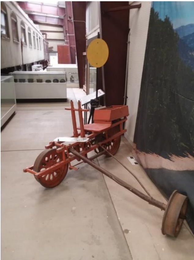
Velocipede used by track workers. It was hand powered by pumping the vertical levers.
